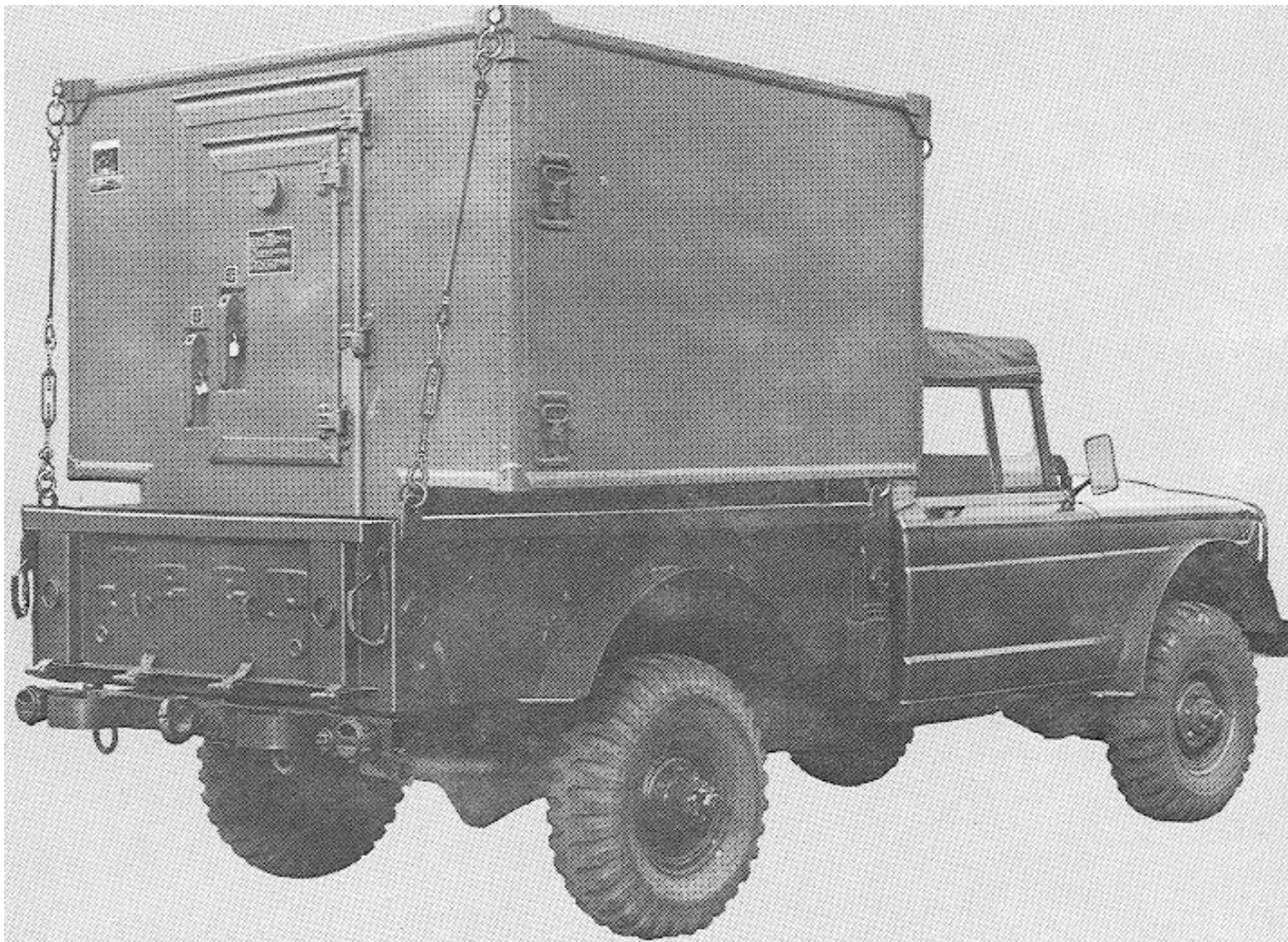
S-250/G Electrical Shelter mounted on M715 Cargo Truck
