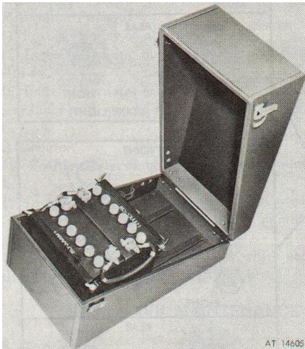
FIGURE 2-38. Batteries, holddown, bolts and straps.
